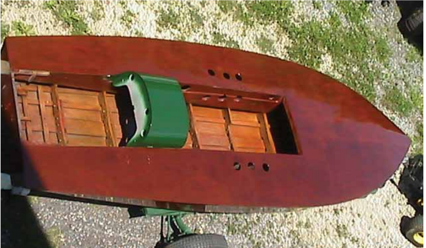
Six coats of varnish, finishing of the painted parts, time to start assembling!
